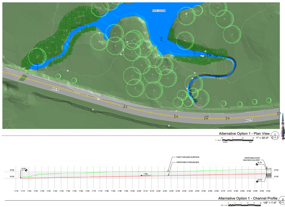
Figure 18 Optional Channel Change proposal showing the Alignment Alternative 1 and the associated Profile.
