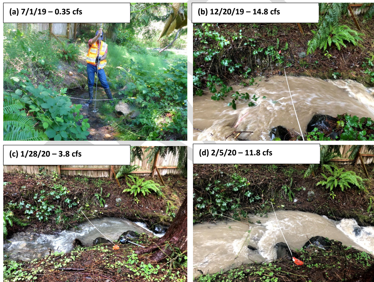
Photo 10. Flow measurements on George Davis Creek
