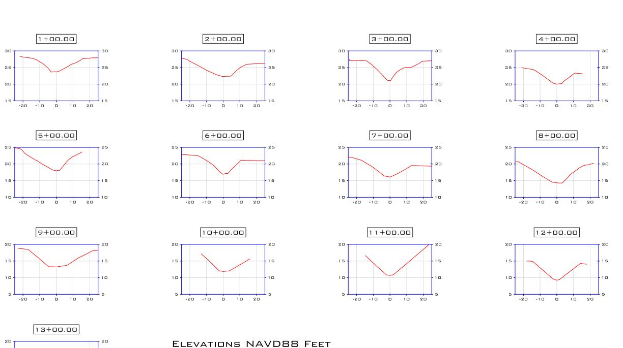
ELEVATIONS NAVD88 FEET VERTICAL EXAGGERATION 2X
