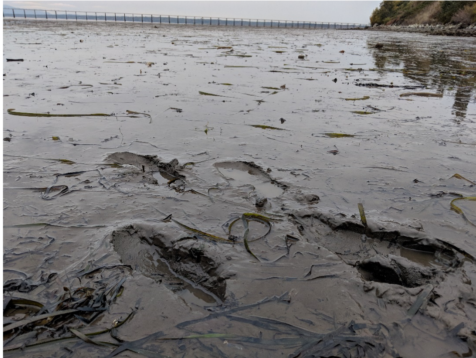
Figure 4: Sunken footprints during a 2018 site visit by a M&N coastal engineer indicate abundance of cohesive fine material on the northwest side of the pier, photo taken between the pier and the supply line looking north.
