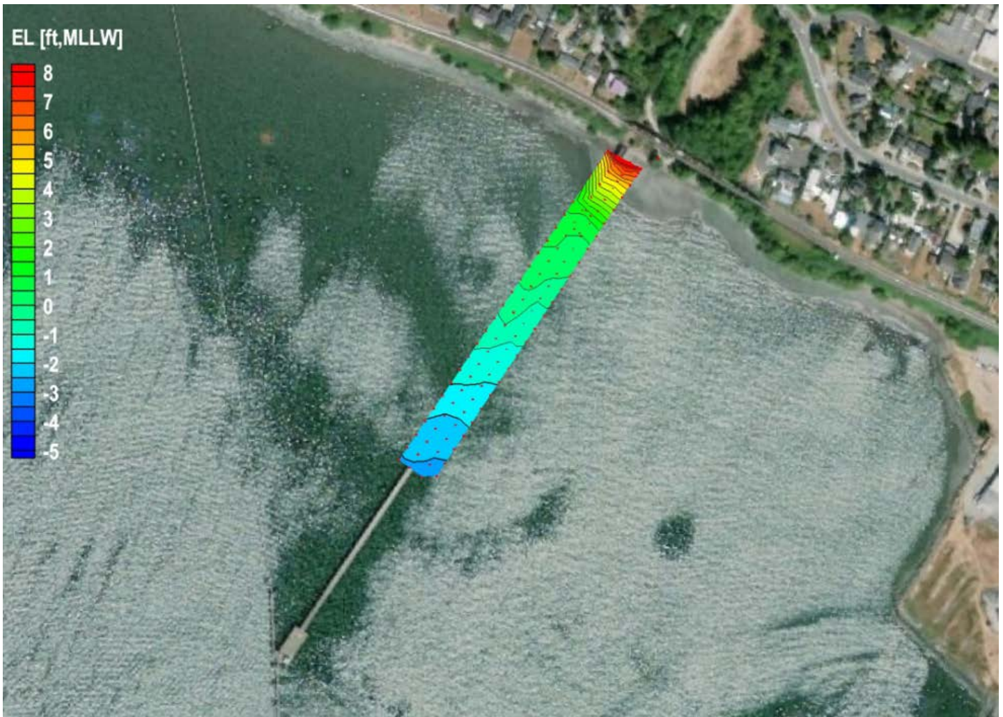
Figure 6: Ground elevation (EL) referenced to MLLW in feet based on a 2018 nearshore survey specifically conducted as part of this project.
