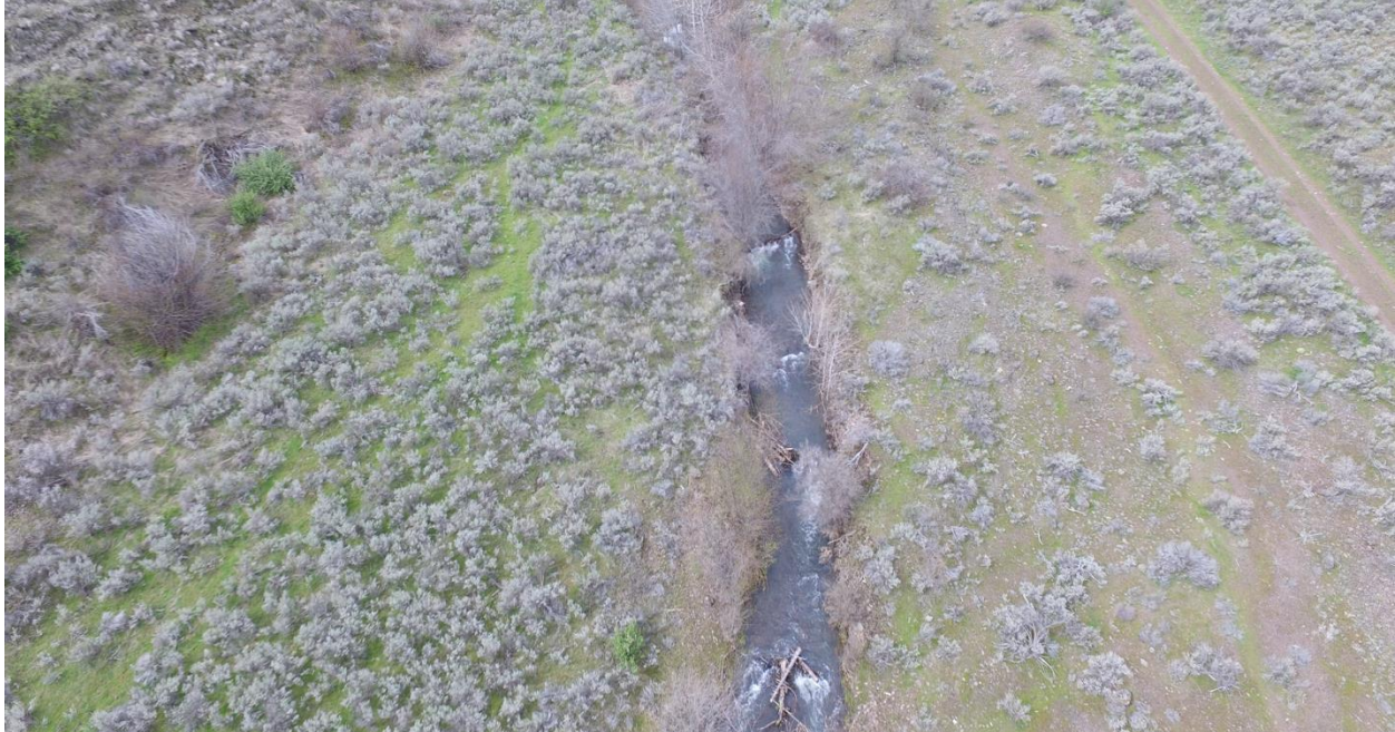
Figure 6. Example of treatment section along Charley Creek where beaver-dam analogs may be used to force floodplain connection during low flows. Post-assisted log structures are increasing hydraulic and geomorphic diversity in Charley Creek but have not forced floodplain connection.
