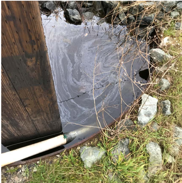
Figure 6: Sheen in water collected in steel casing at the base of utility pole.
