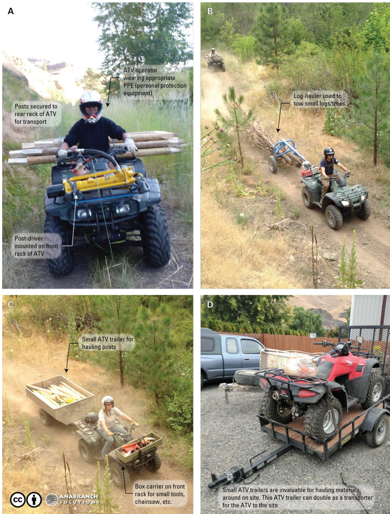
Figure 13 – Where ATV access is feasible, ATVs can be a very handy way of moving materials between staging areas and structure locations.
