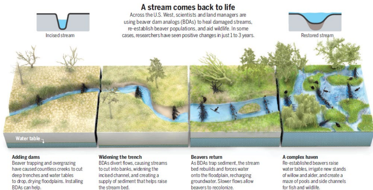
Figure 18 – An example from Goldfarb (2018a) of achieving a self-sustaining condition where meals of beaver dam analogues (BDAs) mimic beaver dam activity, and then the maintenance and expansion of beaver dam activity is taken over by actual beaver, and then they maintain a complex system state. Figure © Science by V. Altounian .
