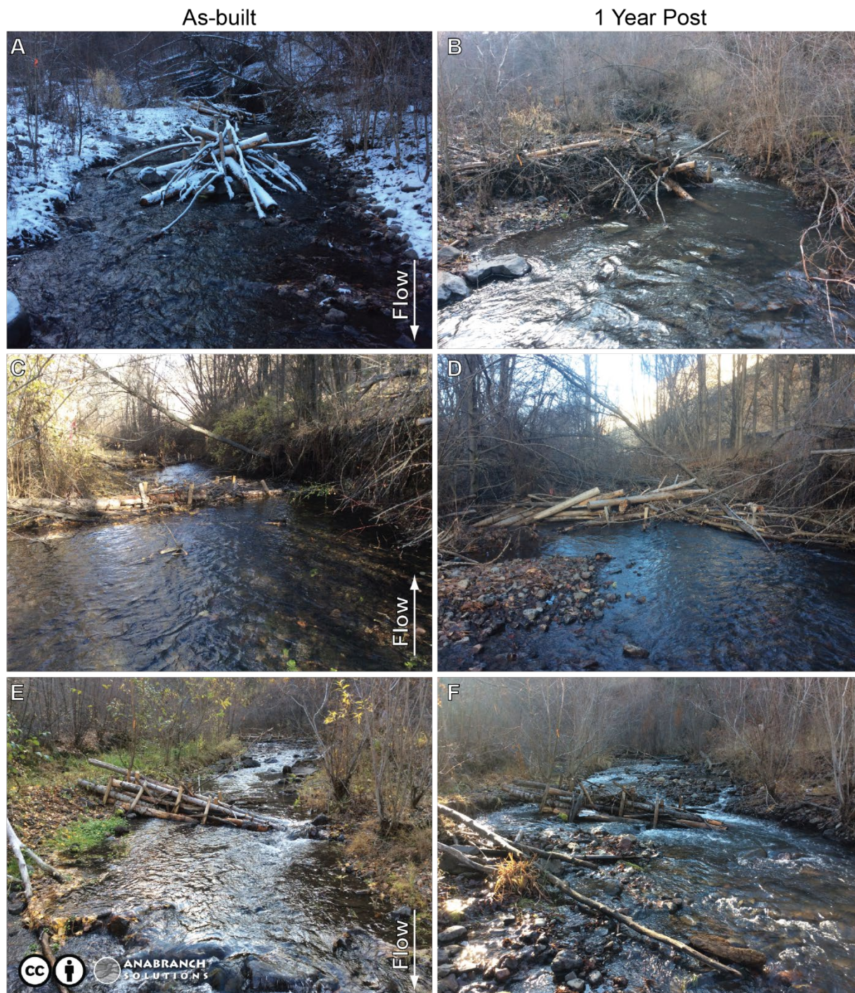
Figure 17. Example of PALS evolution over the course of one year by promoting processes of wood accumulation. A and B show a mid-channel becoming a bank-attached, C and D show a bank-attached becoming a debris jam, and E and F show a bank-attached becoming a mid-channel. The geomorphic changes imposed by the presence of the PALS in each example shows clear alterations to the channel bed and hydraulics.
