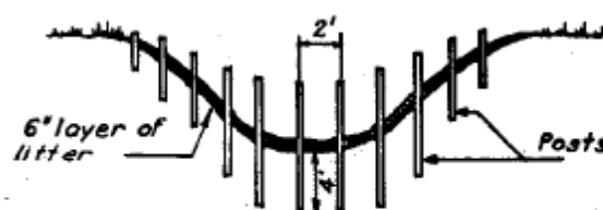
Figure 26 Sectional elevation of gully showing posts and litter in place for dam. Note that the posts are lower in the center.
