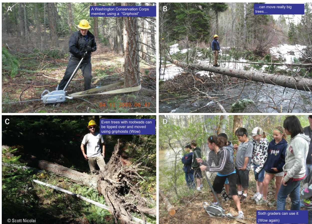
Figure 21 – Griphoists are an effective tool for creating a mechanical advantage and pulling in or over live-trees, dead snags, and/or down trees. A) Example of griphoist being used to pull a tree into a creek. B) A whole tree pulled down across a channel with a griphoist. C) A tree pulled over with its rootwad intact, can be repositioned and dragged into position in a creek. D) When done with supervision and safety in mind, even sixth graders can crank on the griphoist and use the mechanical advantage to move some big material. Slides from Scott Nicolai (Yakama Nations) from a Cheap & Cheerful Restoration Workshop with the Snake River Salmon Recovery Board.
