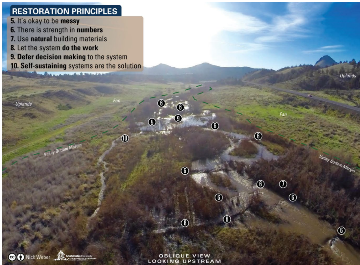
Figure 10 – Illustration of six restoration principles in play, eight years after a restoration treatment. In this reach, roughly 35 beaver dam analogues (BDAs; 9 labeled in photo with “6”), were originally installed in a single-thread channel. Within a year of installation, such a mess was made (5) that the floodplain was experiencing some flooding even at low flow. Other than natural, untreated wooden fence posts, all the building materials were sourced on-site (7). Within months, beaver that were in low numbers in the system opportunistically colonized the BDAs and took over maintenance (8). Within a few years, the beaver extended many of the dams across the valley bottom, effectively converting the valley bottom back to a Stage 0, multi-threaded mess with a highly connected floodplain. Riparian vegetation recruitment has taken off, and beaver now rotate through different complexes in the area (self-sustaining – 9). Now the combination of the flow regime and beaver are making decisions about what parts of the floodplain to flood and when (10).
