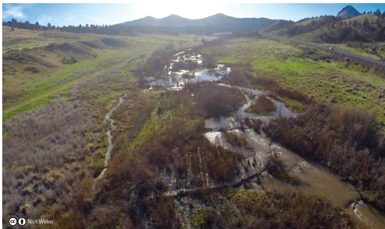
Figure 1 – The vision that guides the use of post-assisted log structures (PALS) and beaver dam analogues (BDAs) is ‘Stage 0,’ where large wood accumulation and beaver dams force the floodplain connectivity, multiple channels and complex physical instream and riparian habitat.
