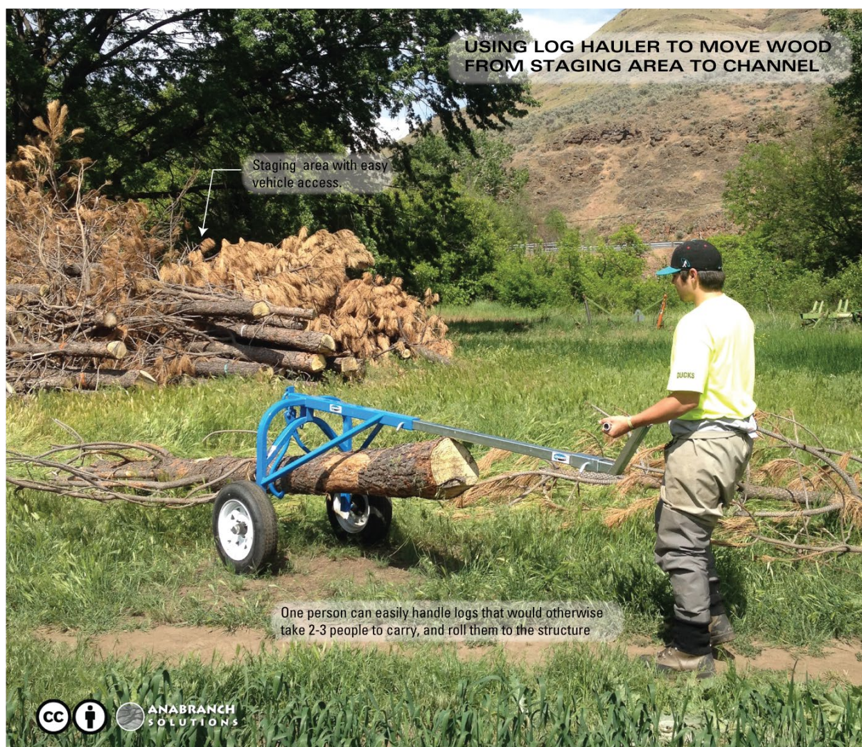
Figure 12 – Hand operated log haulers (e.g., this one is a LogRite Buck Arch ) can make the work of moving 2-guy/gal or 3-guy/gal pieces of wood a one-person job.
