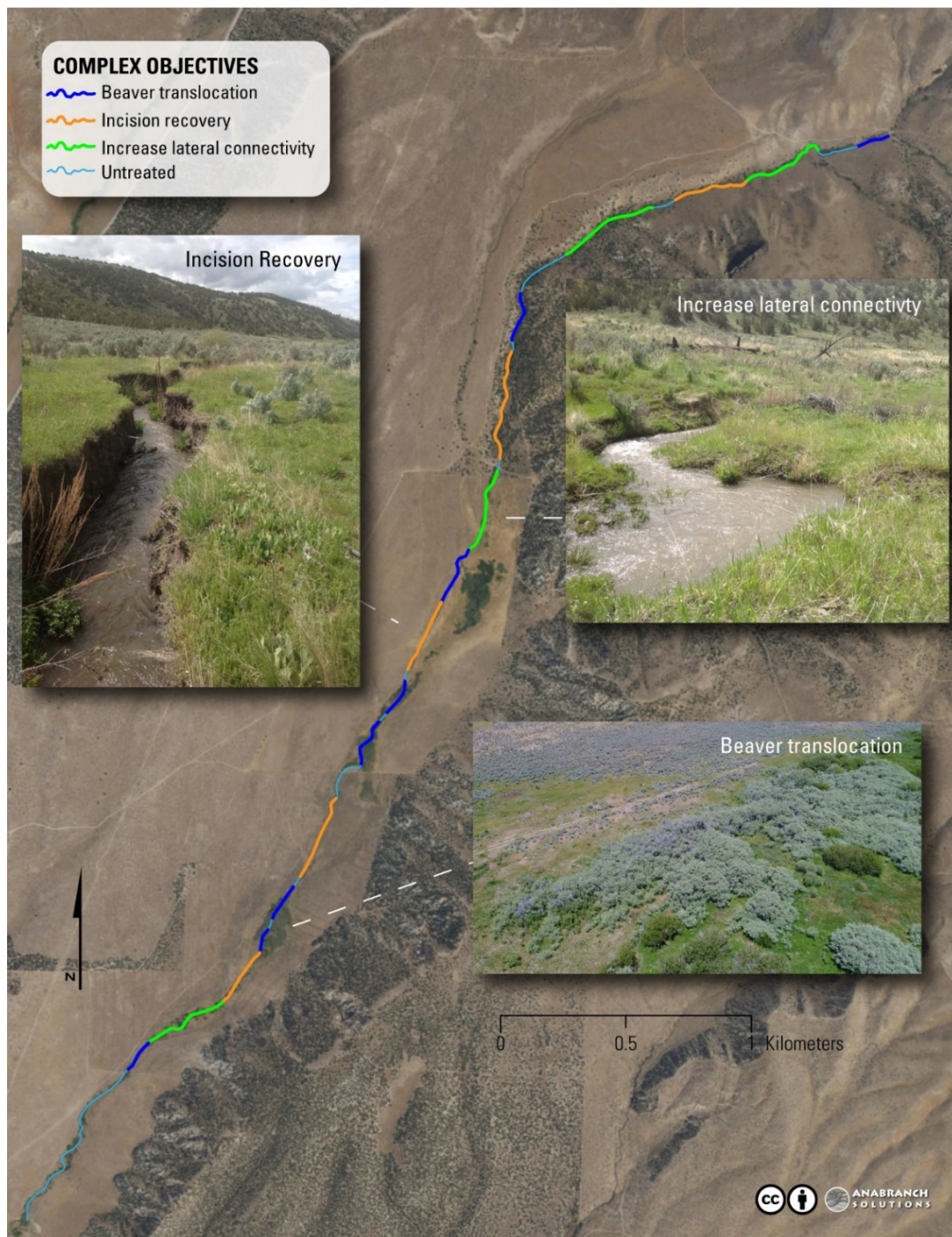
Figure 6 – Conceptual complex design at project scale. The objective of each complex has been identified and is based on reach-scale attributes. Inset photos show different conditions within the project area (total length ~ 4 mi (~6 km) that determine the objectives of each complex. Channel incision (inset left) can be addressed by a complex designed to force channel widening and aggradation. In areas with accessible floodplain but no woody riparian vegetation (inset, top right) complexes can restore immediate channel-floodplain connectivity. Areas with abundant woody riparian vegetation (inset, bottom right) are suitable for beaver translocation and complexes can be designed to create immediate deep-water habitat for translocation. Complexes are represented as lines rather than points to better depict their longitudinal extent on the channel network. When mapping at higher resolutions, we recommend mapping complexes as polygons to represent their anticipated hydraulic zone influence Figure 8 and Figure 9 . Note that complexes may or may not be adjacent to one another, such that one complex begins where another ends. Furthermore, two complexes with the same goal may be adjacent to one another. The specific types and locations of individual structures is necessarily determined in the field.
