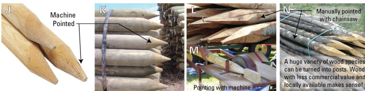
Figure 4 – Posts are used to provide temporary stability or pins when building many low-tech restoration structures (e.g., post-assisted log structures). Many commercially available fence post options are available, but a premium price is charged for consistency, larger diameter, and straight poles (e.g., peeler cores and lodge pole (A, G, J, K). Rough logs (C, N), smaller diameter tree stakes (H, I) are cheaper, and often available from fuels reduction (F) or non-commercially viable slash from timber harvest operations. Since posts are driven into substrate, they need to be pointed at tips (A, E, H-N). Pointing can be done by supplier (typically with a machine – e.g., M) or by an experienced chainsaw operator with four cuts (L & N).
