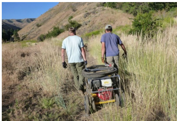
Figure 17 - Moving the power pack (Atlas LP 13-20) and hose that drives the hydraulic post driver is at least a two-person job if it can be rolled, and is often easier with three or four. It typically takes three to four people to lift and/or carry it short distances.
