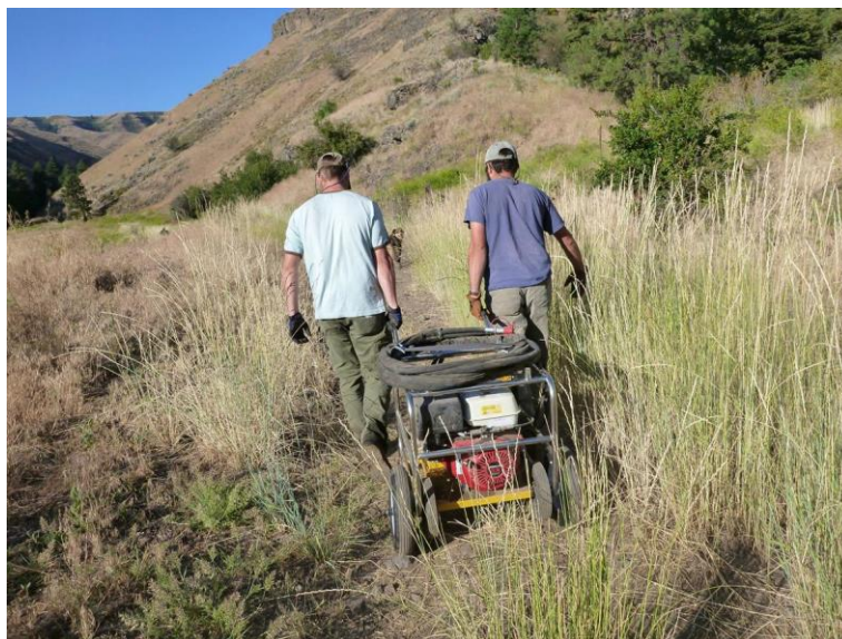
Figure 43. Example of the hydraulic power unit used to power the post driver for installing DWS in the Asotin Creek Watershed.
