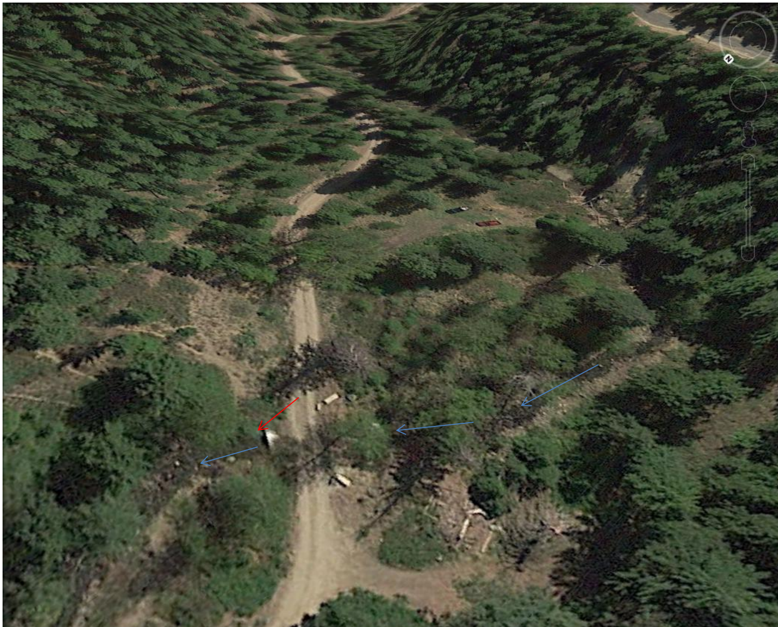
Figure 2: Google earth oblique image of the project area (May 2015). Note the angle of the culvert crossing is not perpendicular to flows. Blue arrows depict stream flow. Red arrow depicts overland flow due to channel constriction. Overland flows are eroding/comprising the current structure and causing increased fine sediment deposition to the stream.
