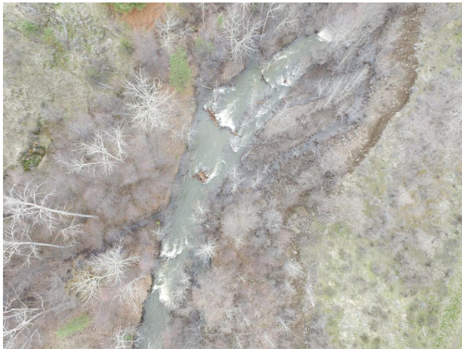
Figure 11. South Fork Asotin Creek treatment section 1 in the spring of 2017 overflowing the banks and reconnecting with the floodplain. We had not observed overbank flow in the South Fork since the IMW started in 2008. Note the high-density of large woody debris that is causing the response.
