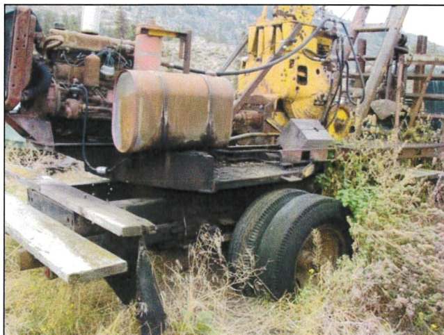
Photo F-37: This photo is of a mounted engine and fuel tank that appears to have had some leaking that was observed in the bone yard area.
