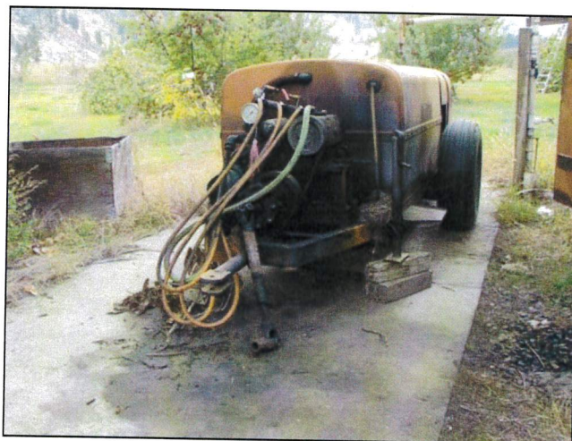
Photo F-15: View an orchard heater that is parked directly in front of the pesticide shed. There is oil staining from the heater on the concrete pad and in the gravel off to the right.
