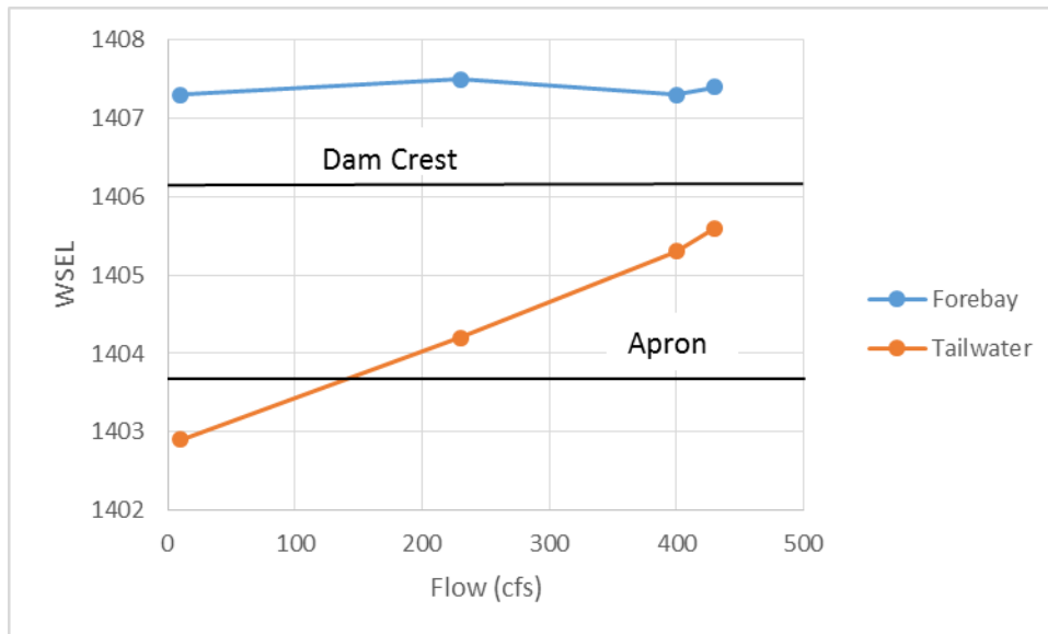
Figure 11 – Forebay and tailwater rating curves for the concrete diversion dam on Icicle Creek. The apron is concrete and broken at the downstream end.
