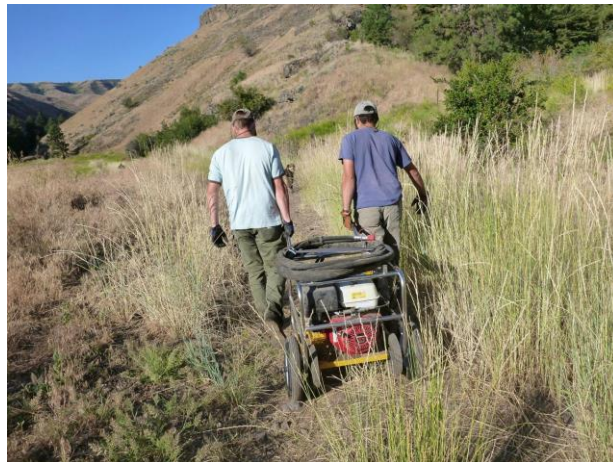
Figure 15. Example of the hydraulic power unit used to power the post driver for installing DWS in the Asotin Creek Watershed.
