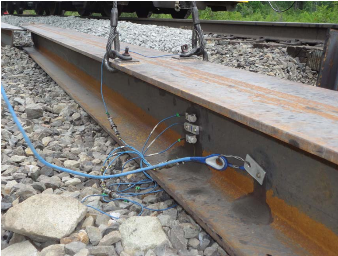
Photo 1: View of the pile driving analyzer equipment that was attached to BNSF's follower.
