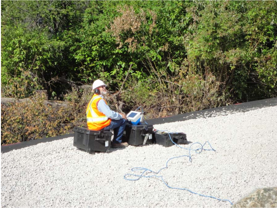
Photo 3: View of the computer Bert had setup to collect pile driving data.
