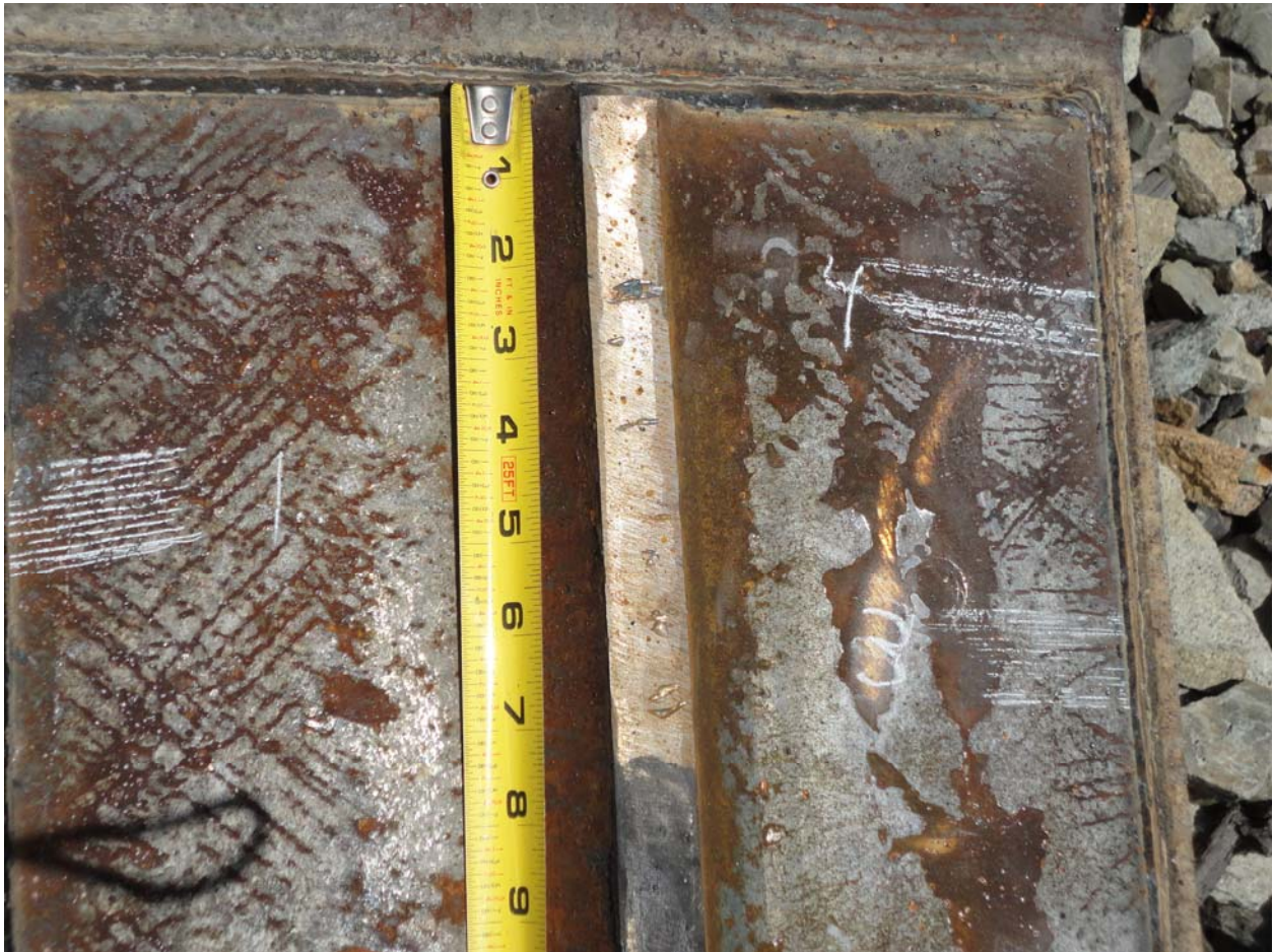
Photo 1: View of the restrike marks that were made on the follower from Pier 3, piles 1, 3, and 4.
