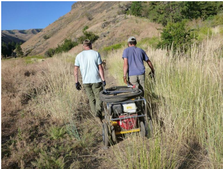
Figure 8. Example of the hydraulic power unit used to power the post driver for installing DWS in the Asotin Creek Watershed. The post driver can be manipulated by two people and has a 25 m hose connected to a gas engine power unit. The driver weighs approximately 30 kg and the power pack weighs approximately 75 kg. The power unit has large rubber wheels to improve transport over rough terrain. The power unit can also be carried by 2-4 people when the terrain is too rough for wheeling.
