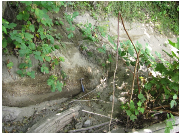
Reference bluff 4 – sand and pebble with minor toe erosion
