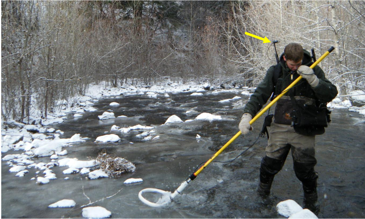
Figure 23. Mobile PIT tag survey setup including custom antenna, GPS unit, data logger and PIT tag reader used to resight PIT tagged fish in the Asotin IMW study streams. Arrow is pointing to GPS receiver.
