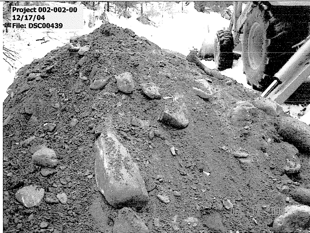
Photograph 3. Photo looking at soil excavated from a depth of approximately 4 to 5-1/2 feet in Test Pit 1. Large 1 to 2 foot cobbles became more abundant at approximately 4-feet.
