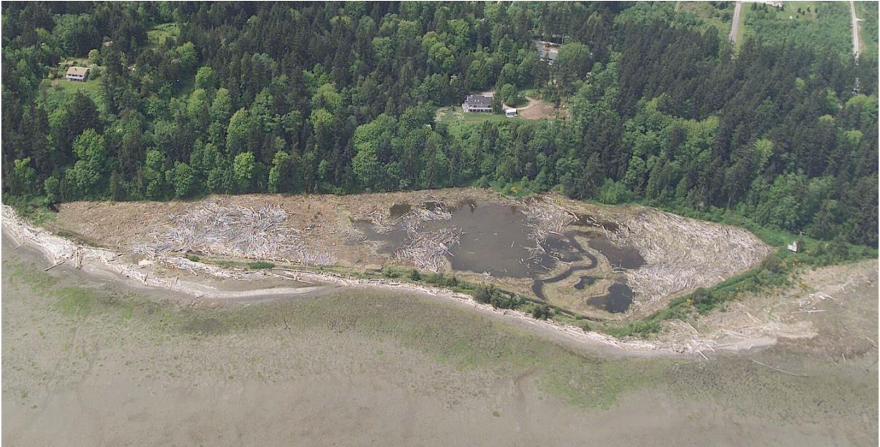
Figure 3 Aerial photo of the restoration site taken in 2011 (after the breach in the southern portion of the dike). Large amounts of wood carried in during storms and high tide events piled up in the interior.
