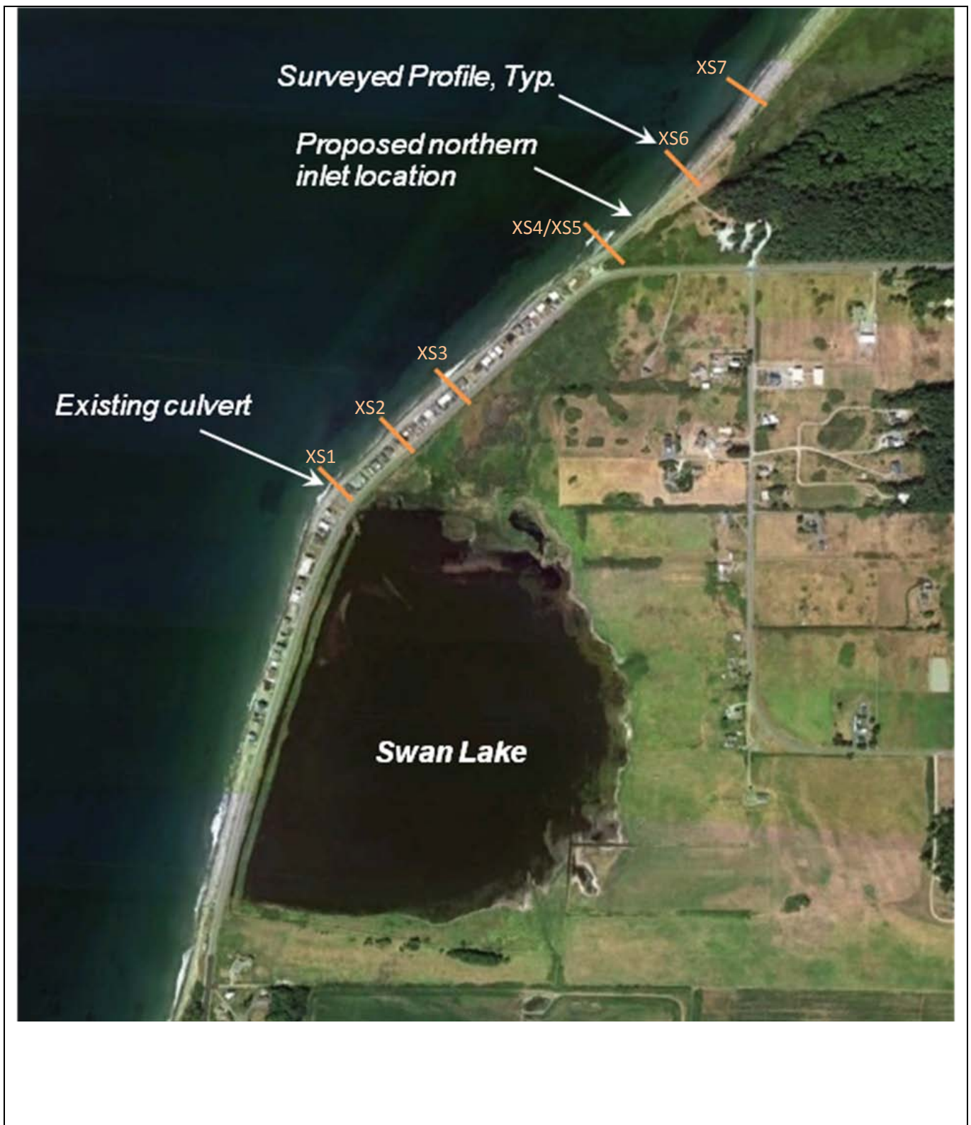
Figure 2 Site Map of Swan Lake showing the location of the existing culvert and proposed Northern Inlet site
