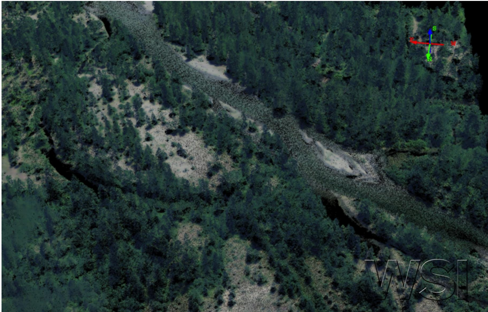
Figure 15. 3D point cloud colored by RGB values extracted from 2009 NAIP imagery, looking south over the Cle Elum River
