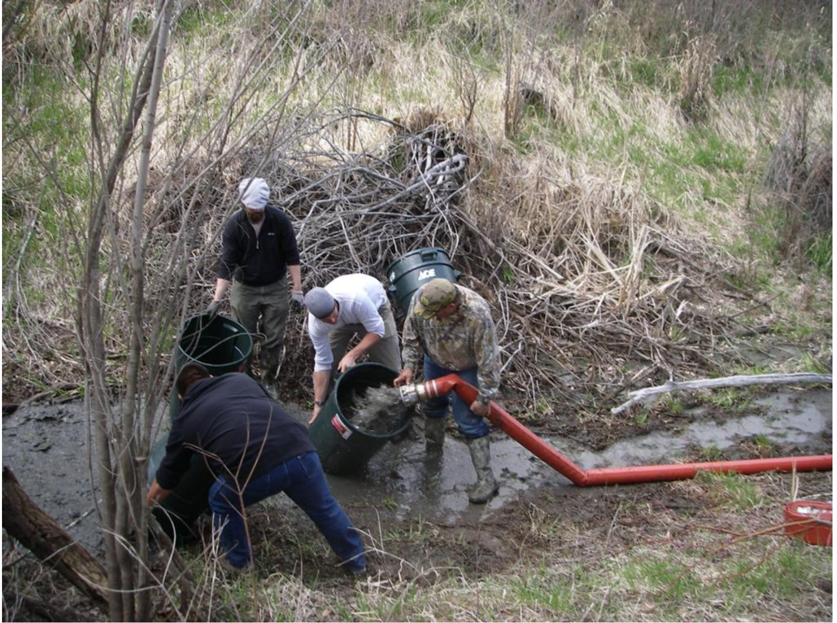
Draw-down/recharge ground water testing (west/Similkameen channel). Preliminary results are positive.
