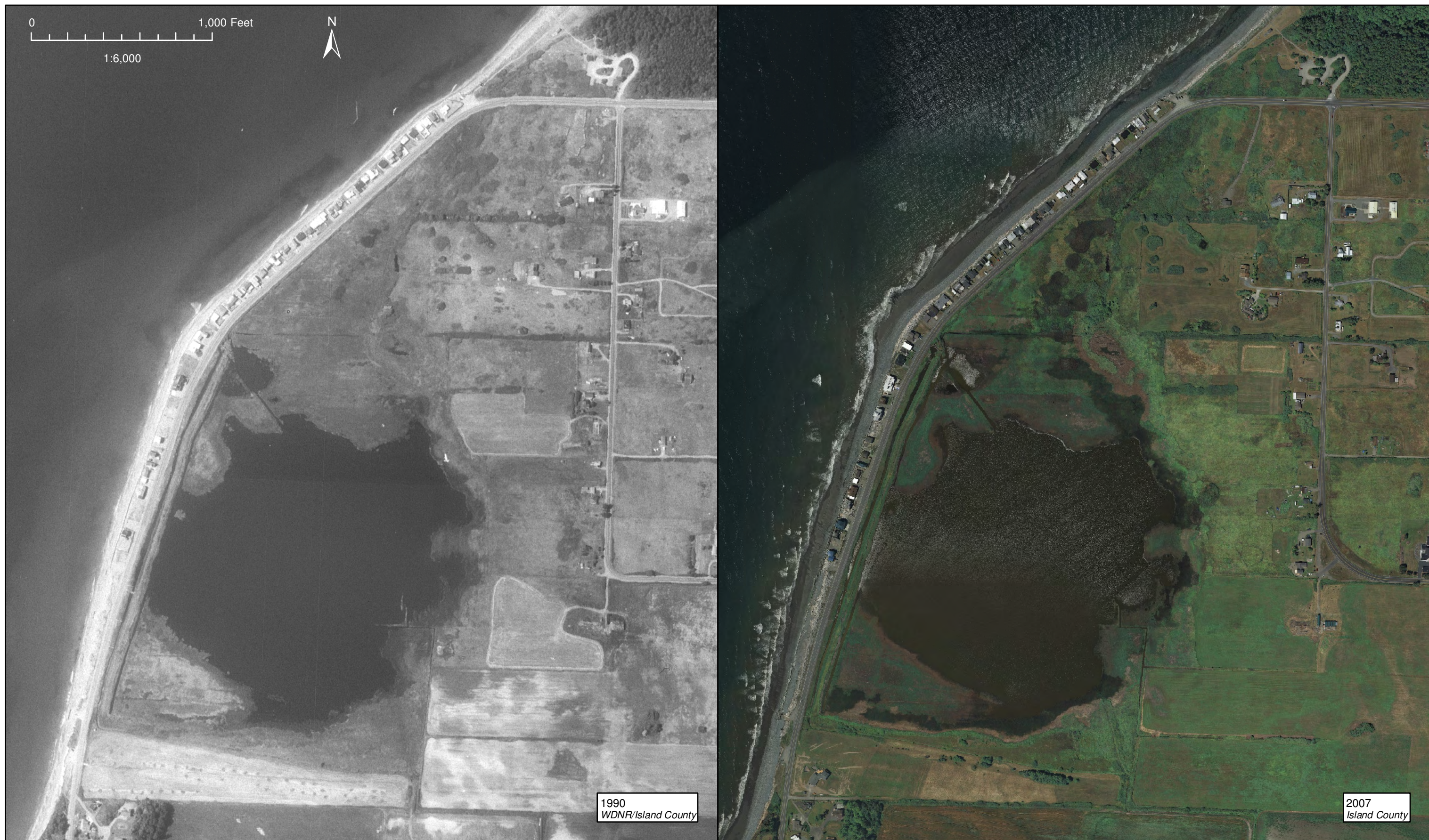
Figure 6c. Aerial photographs from 1990 and 2007. Note the high water level in 1990 and 2007, likely due to lack of tide gate maintenance following dissolution of Drainage District No. 1. 2007 water level was on the order of +2 to +3 ft MLLW based on field survey.
